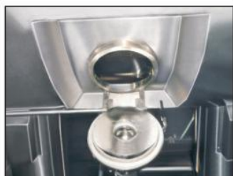
Flush discharge gate
